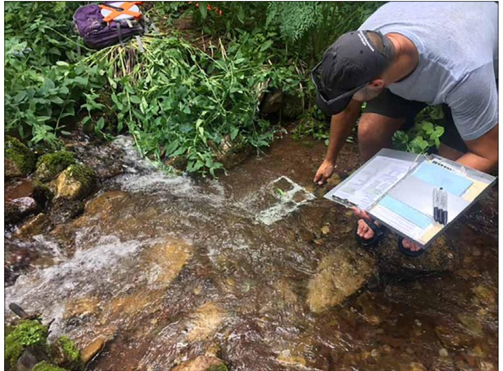
*A device called a "gravelometer" (shown in the water) is used to measure the size of sediments (pebbles, cobbles, etc.) found in the stream banks and bed. This is one of many data variables collected by the Watershed Program to assess stream channel stability.*
